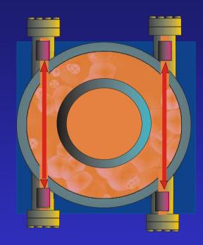
Sound path without reflection on the drill pipe
